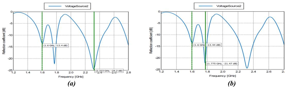
Figure 4. Simulated result for Return Loss (a) at 1.6GHz and 2.32GHz (b) at 1.6GHz and 1.775GHz
