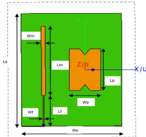
Figure 2. Design geometry of coplanar integrated microstrip antenna for GPS, GSM and LTE2300 applications
