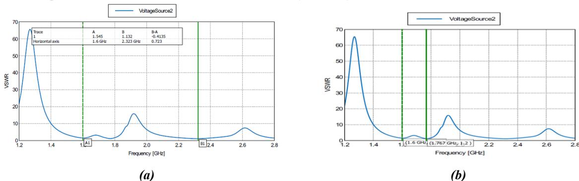
Fig 5. Simulated result for VSWR (a) at 1.6GHz and 2.32GHz (b) at 1.6GHz and 1.775GHz
