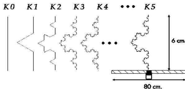
Figure 3. Iterative construction of Fractal Koch curve
