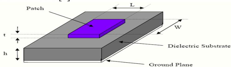
**Figure 1. Structure microstrip patch antenna**
