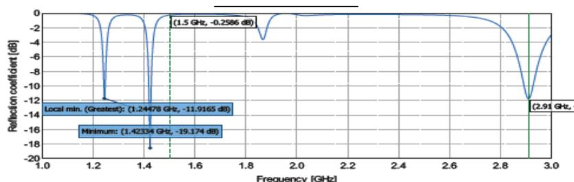
Figure 6. Reflection coefficient Magnitude [dB] – Fractal TMSA Iteration 2
