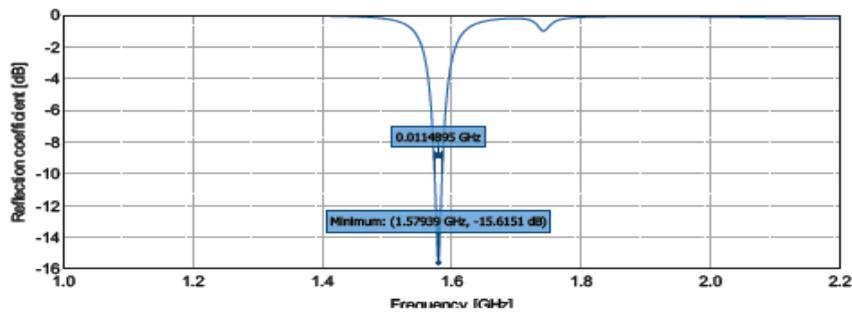
Figure 4 . Reflection coefficient Magnitude [dB]-Fractal TMSA Iteration 0
