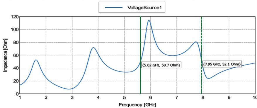
Figure 8. Impedance Magnitude [Ohm] – Final Suspended Fractal Antenna
