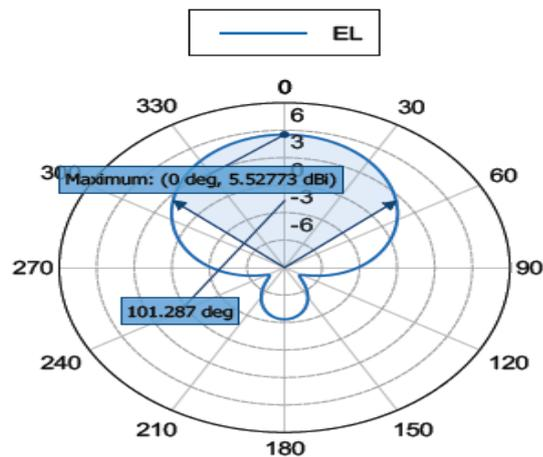
Figure 9. Total Directivity [dBi] (Frequency = 1 GHz; Phi = 90 deg) – Final Suspended fractal Antenna
