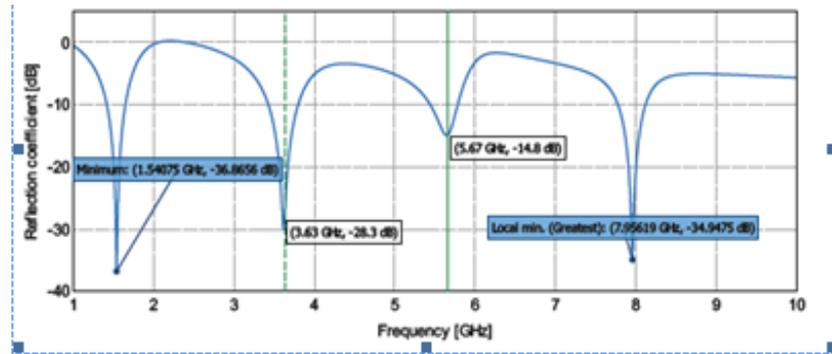
Figure 7. Reflection coefficient Magnitude [dB]- Final Suspended Fractal Antenna
