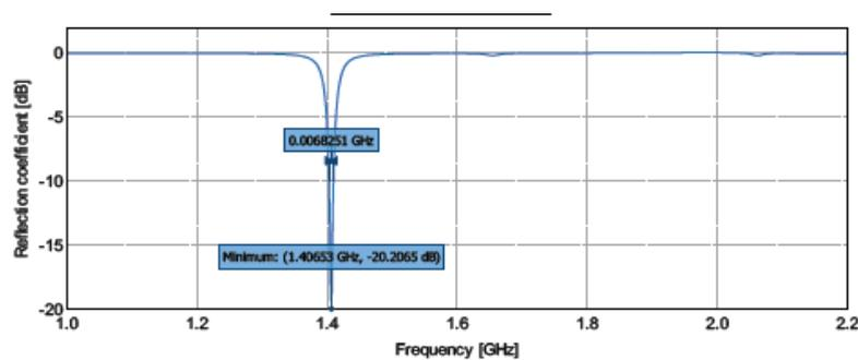
Figure 5. Reflection coefficient Magnitude [dB] – Fractal TMSA Iteration 1
