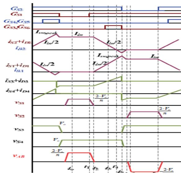
Figure 3. Operating waveforms of proposed ZCS current-fed converter
