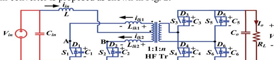
Figure 2. Proposed push-pull DC/DC converter
