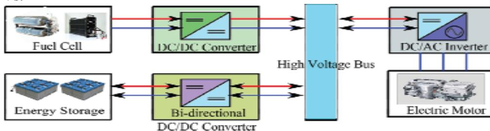
Figure 1. Diagram of a FCV propulsion system
