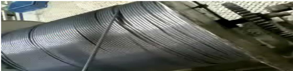
Fig 1- Bobbin feeding misalignment due to improper winding
