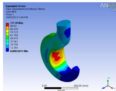
Figure 8. Stress pattern for Optimized cross-section
