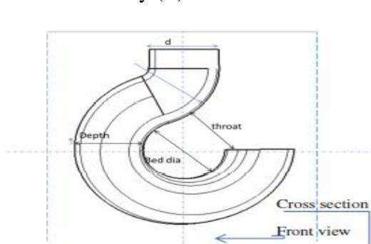
Figure 1. Basic dimensions of crane hook
