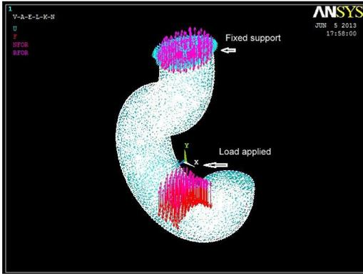
Figure 3. Boundary conditions for crane hook
