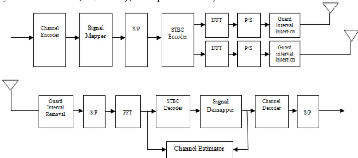
Figure 1. Proposed STBC-OFDM system with two transmits antennas and one receive antenna.
