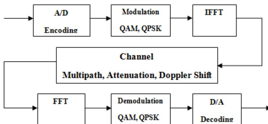
*Figure 2. OFDM Block Diagram*
