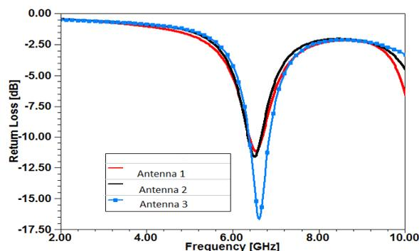
*Figure 2. Simulated return loss of Antenna 1–3.*
