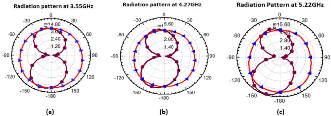
Figure 5. Simulated Radiation Pattern at 3.55, 4.27, 5.27 GHz. Red curve is for yzplane vertical cut and purple curve is for xyplane horizontal cut w.r.t patch lies in xyplane
