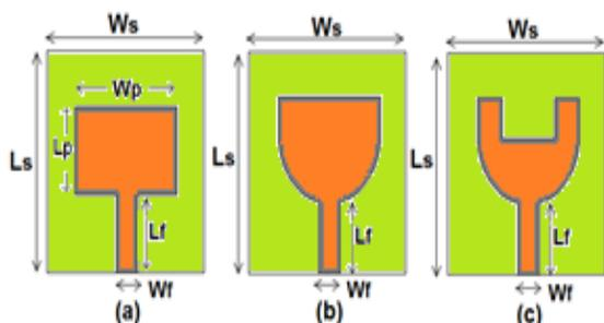
*Figure 1. Different shapes of patch of UWB antenna*
