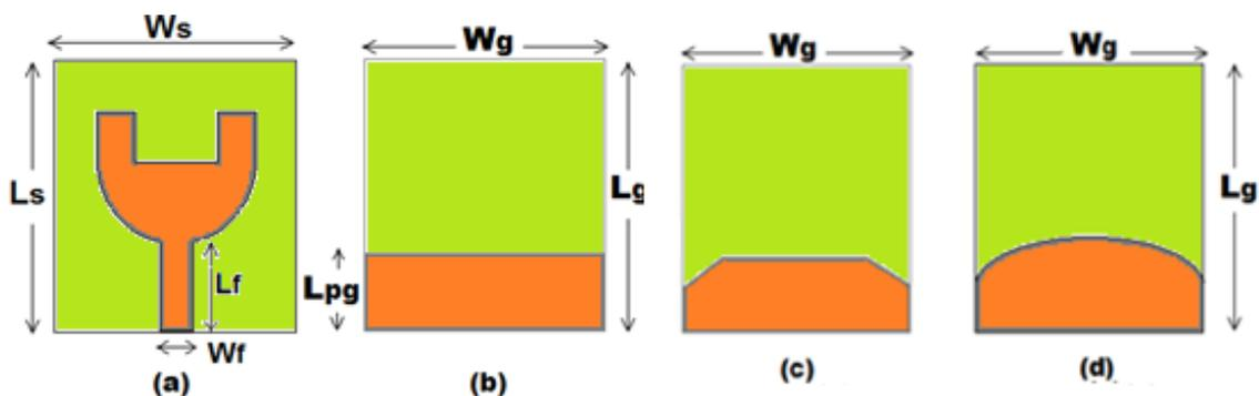
Figure 3. UWB antenna with various Ground Shape
