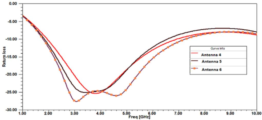
Figure 4. Simulated return loss versus frequency plots of Antenna 4-6.
