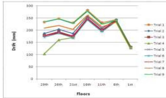
*Figure 2. Drift in X direction for all trials of Model 6.*
