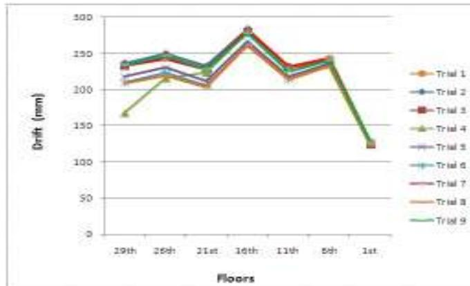
*Figure 3. Drift in Y direction for all trials of Model 6.*
