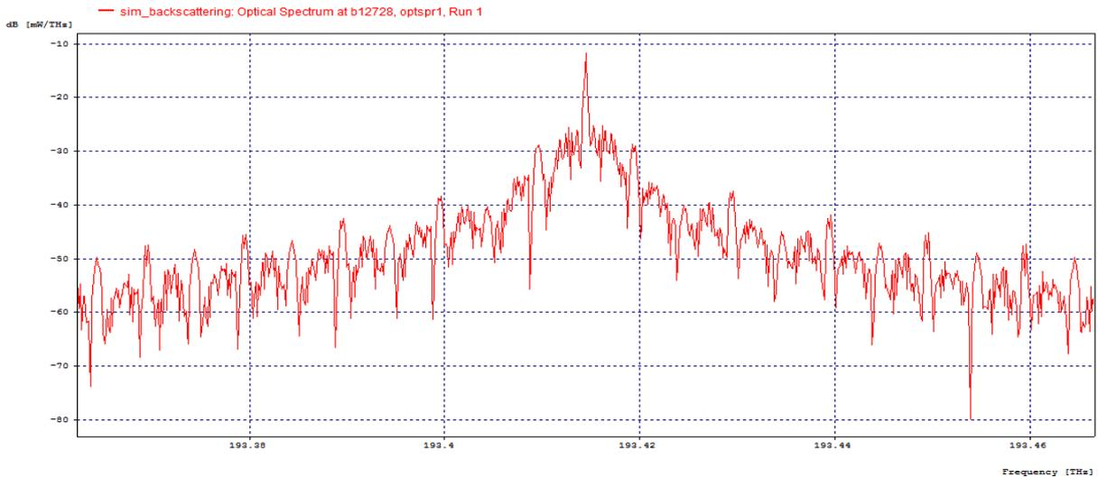
Figure 3. Optical spectrum for VCSEL
