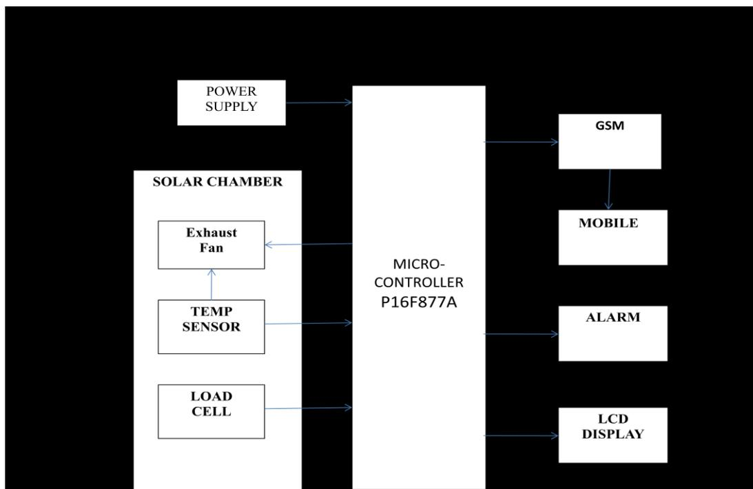
*Figure2. Block diagram of solar dryer*
