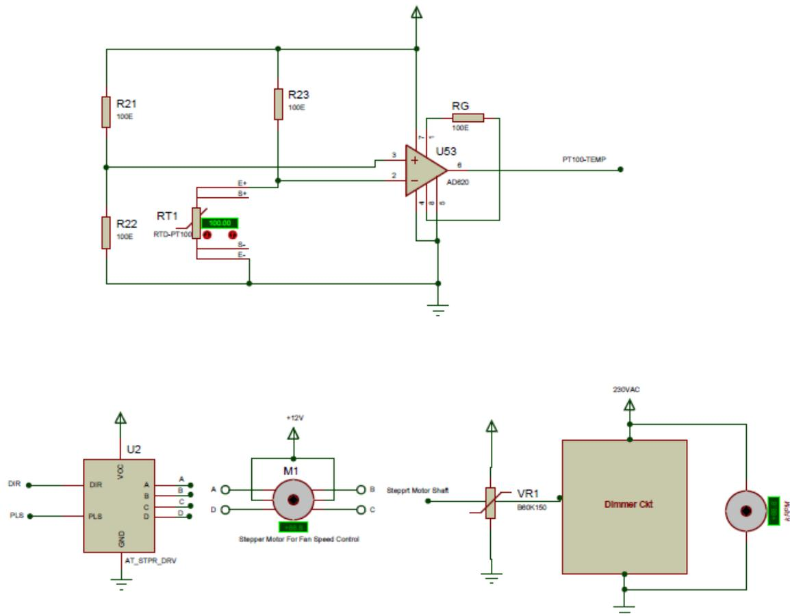
**Figure4. Interfacing of PT100 and fan with controller**
