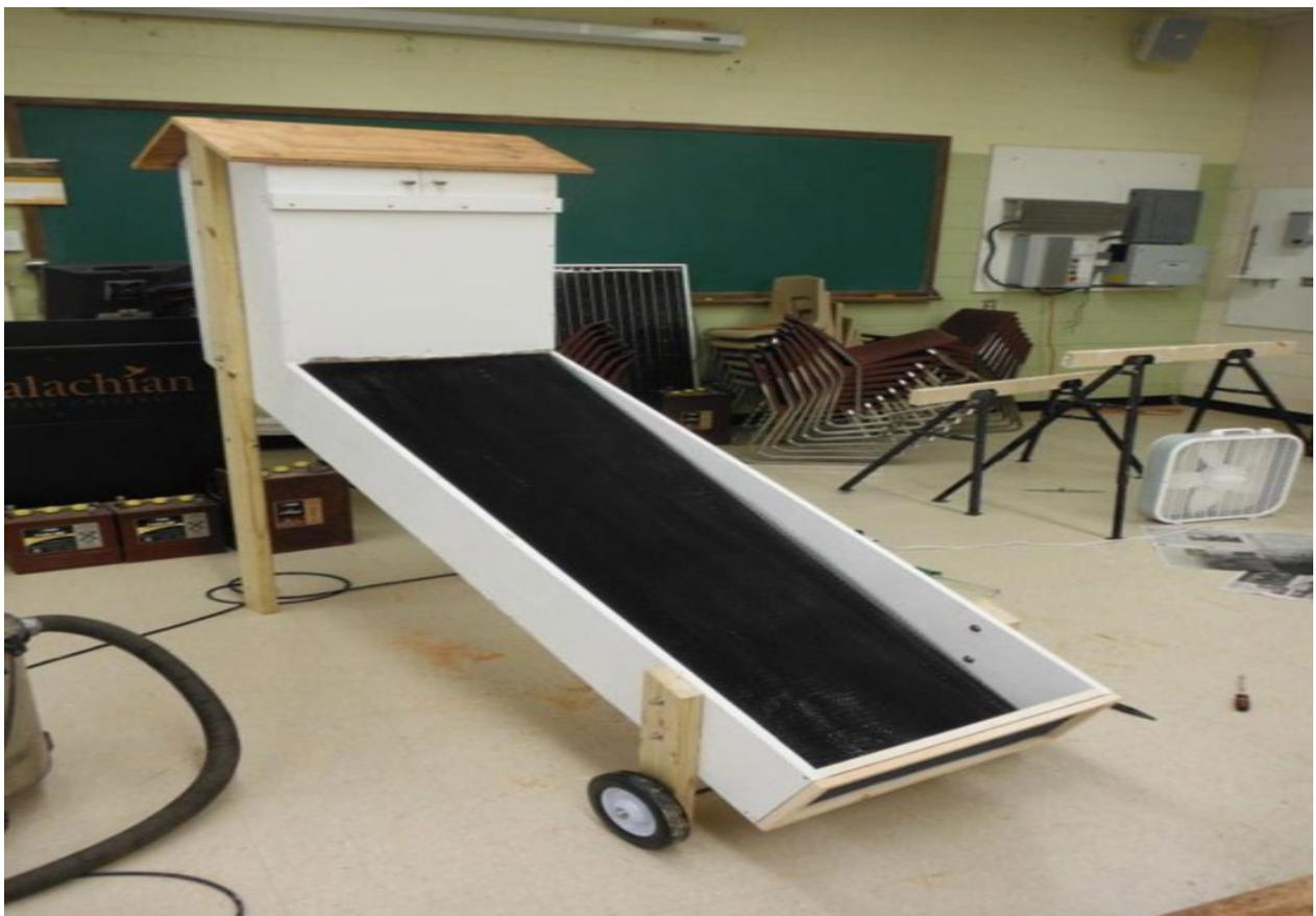
*Figure1. Solar cabinet dryer*
