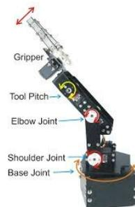
**Figure 3. Four Axis Robot Arm**
