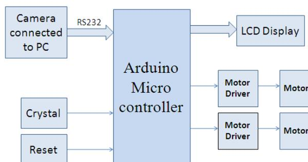
*Figure 2. Block Diagram of System*
