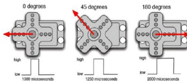
**Figure 4. Servomotor Rotation**
