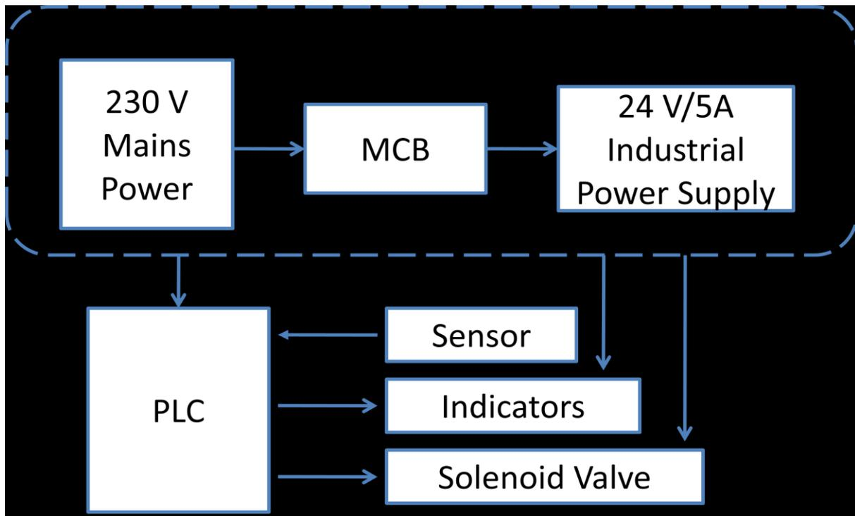
Figure 3. Electrical Signal Flow Diagram
