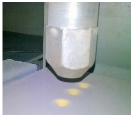
Fig. 2 AJM nozzle erosion
