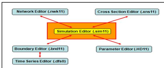
Figure 5. Files to be attached in Simulation Editor
