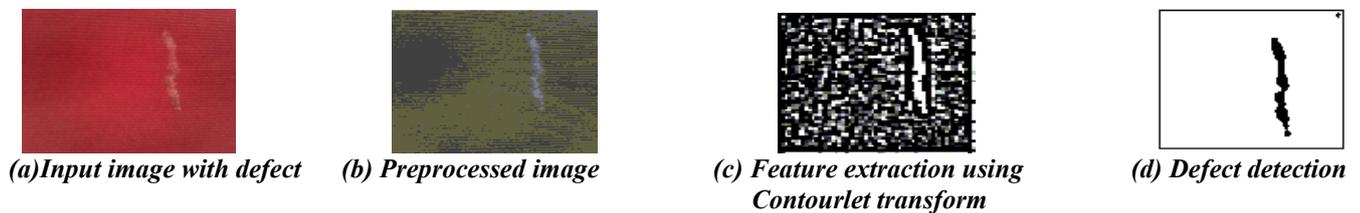
*Fig. 2 Fabric defect detection of the acquired input image*
