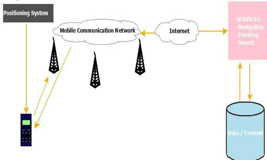
Figure 1: LBS components and Service Process
