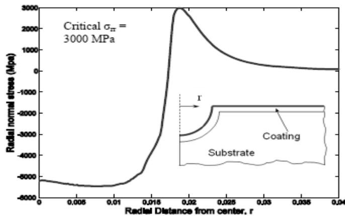
Fig. 1. Distribution of stresses during indentation in benchmark model Radial normal stress along coating surface
