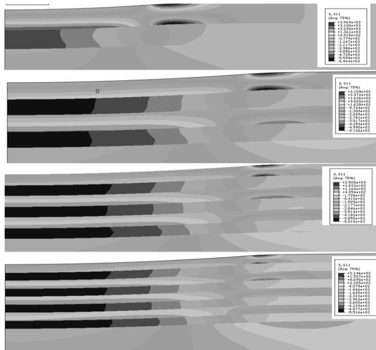
Fig. 3: Contour plots of normal radial stresses for (a) 2 layer, (b) 4 layer, (c) 6 layer and (d) 8 layers
