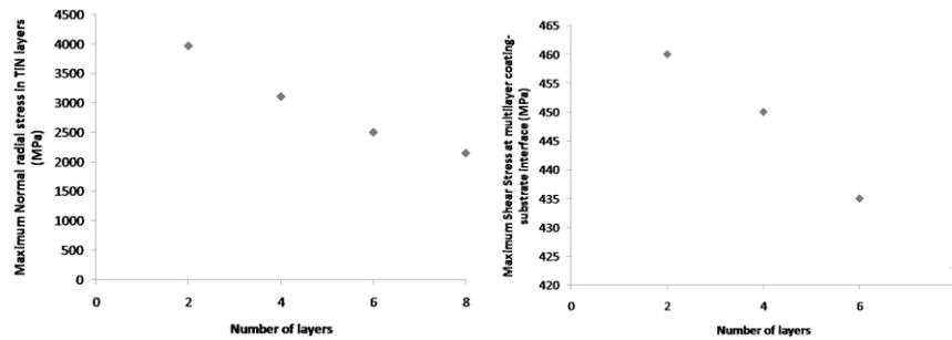
Fig. 5: Variation of maximum radial normal stresses and shear stresses with change in number of layers for the same overall thickness
