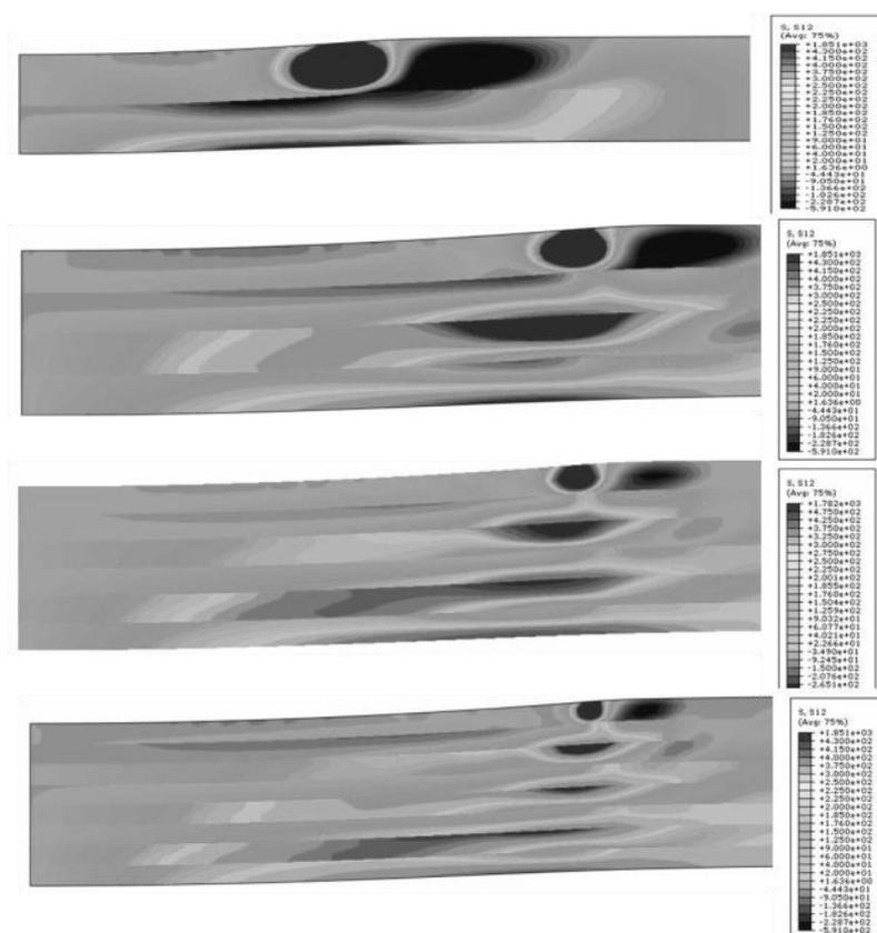
Fig. 4: Contour plots of shear stresses for (a) 2 layer, (b) 4 layer, (c) 6 layer and (d) 8 layers
