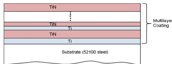
Fig. 2. Schematic of multilayer coating architecture consisting of alternating TiN and Ti Layers
