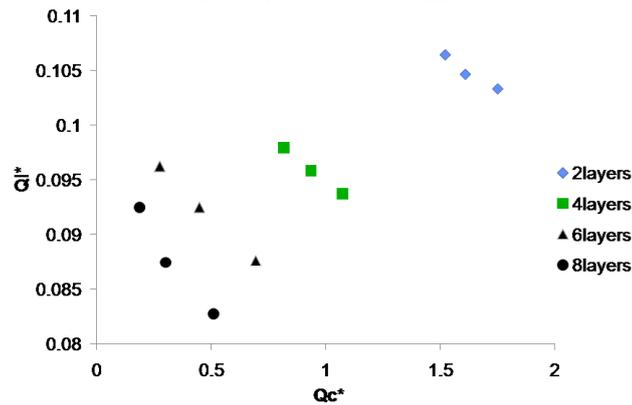
Fig. 6: Variation of damage initiation parameters for different number multilayer designs
