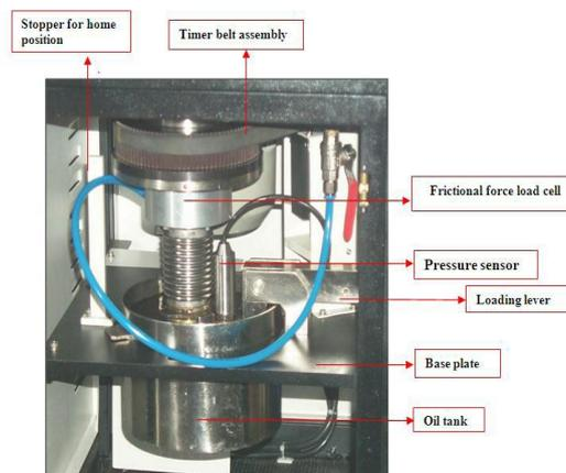
Maximum pressure (kpa) reading at given load is to be noted. Three to four readings should
