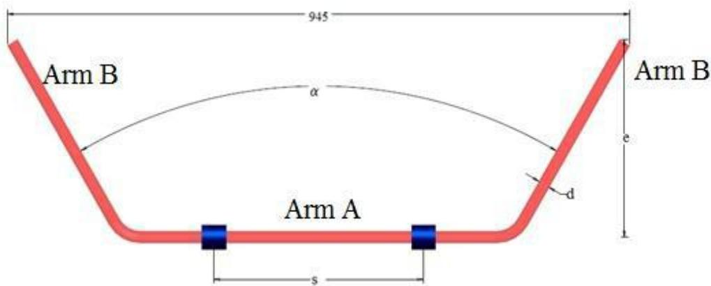
Fig 2: Parameters of Anti-roll bar
