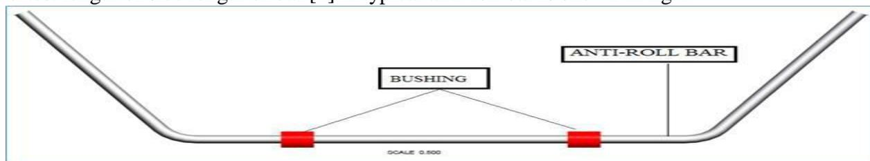
*Fig1: Typical Anti-roll bar with bush*
