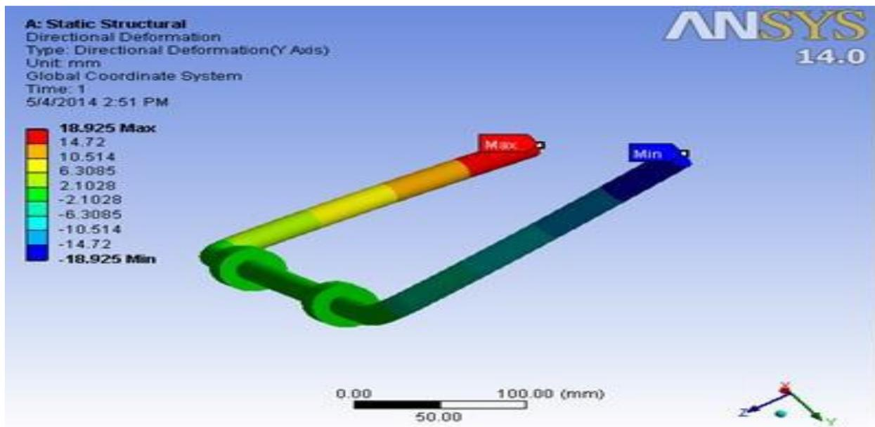
Fig 3: Deformation in Anti-roll bar
