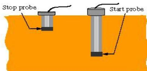
*Figure1. Automatic Moisture Control using two probes: Start & Stop probe*
