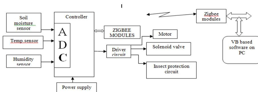
Figure 2. Block Diagram for proposed Irrigation System
