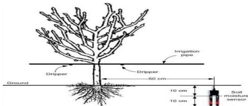
*Figure 3. Location of the Soil Moisture Sensor in this Application*
