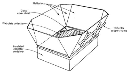
Fig 3. Collector solar cooker
