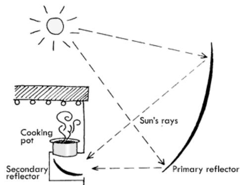
**Fig. 9.** Arrangements of Standing Dish with Secondary Reflector Indoor Cooking
