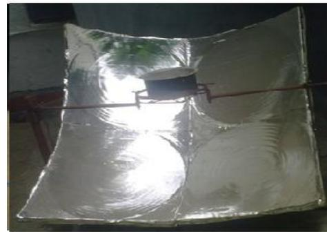
**Figure 6.** PRINCE-15 Fabricated Solar Cooker    **Fig 7.** PRINCE-15 Segmented Solar Cooker.
