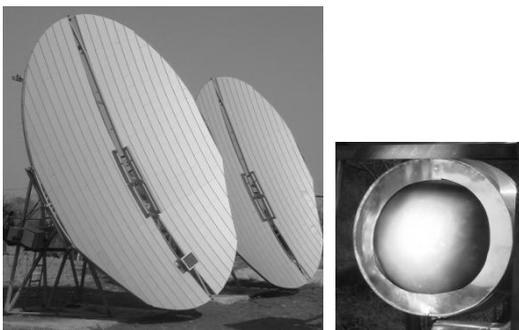
**Figure 10.** Standing Scheffler primary and secondary reflectors
