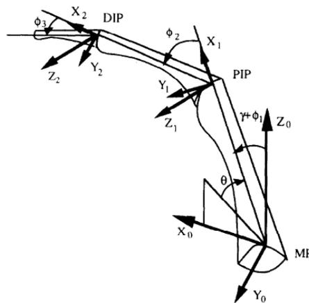
*Figure 1. Mechanical assembly of index finger*
