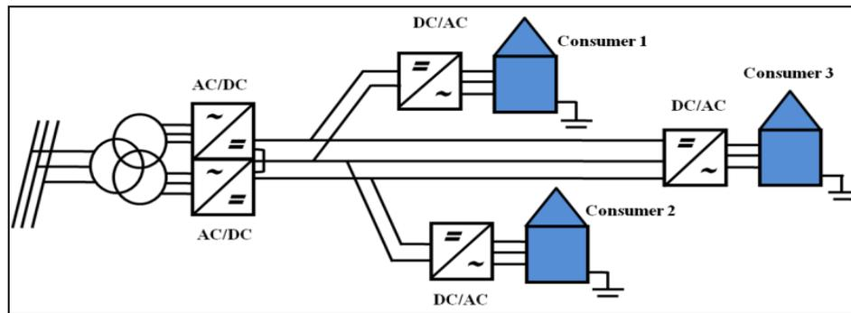
Figure 2. Bipolar LVDC distribution system with different customer connection alternatives
