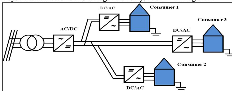
*Figure 1. An unipolar LVDC distribution system*
