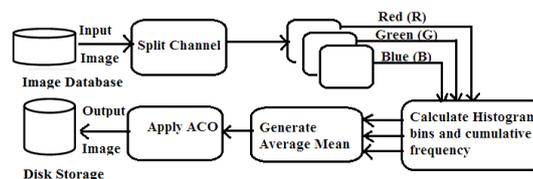
Figure 2. Block Diagram of Proposed System
