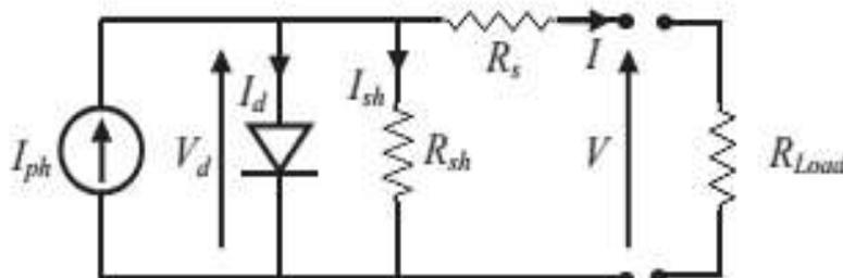
Fig. 2 Typical circuit of PV solar cell
