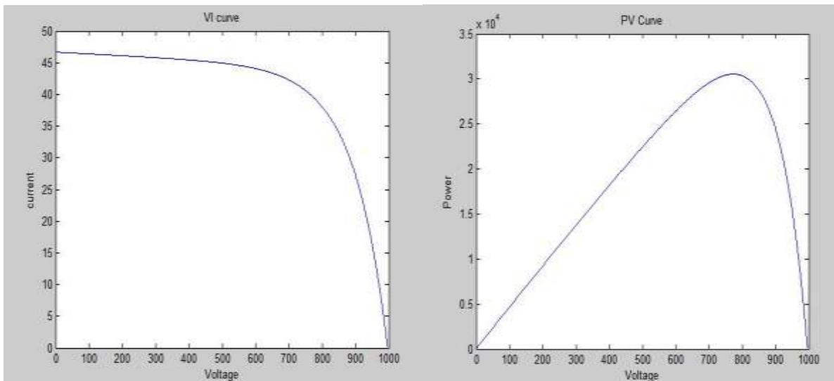
Fig .6 IV & PV curve of Photovoltaic cell
