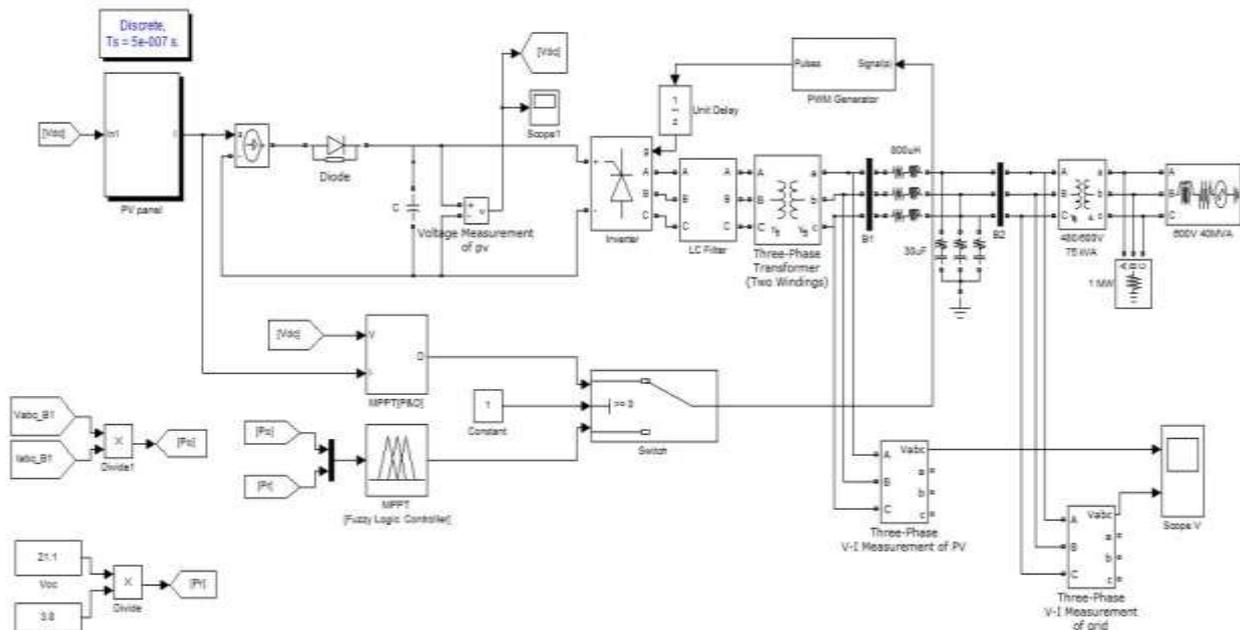
Fig. 5 Proposed grid connected Simulink model
