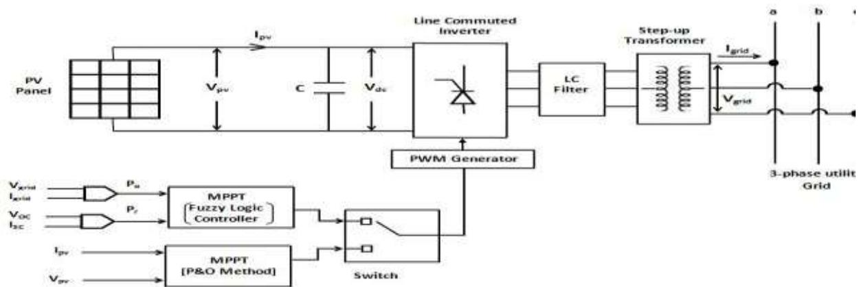
Fig. 4 Basic PV system integrated with 3-Phase Utility grid
