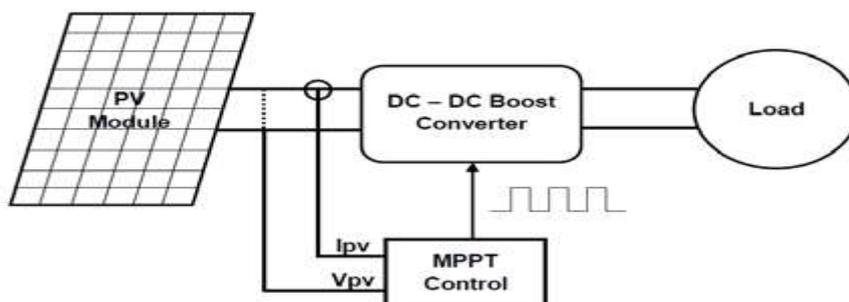
Fig. 1 Typical diagram of MPPT in a PV System
