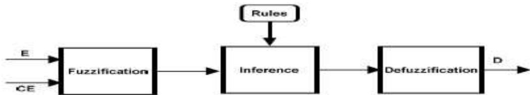
Fig. 3 The Fuzzy Logic Controller
