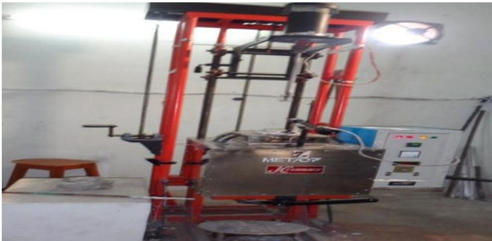
Fig 1: Bottom pouring Furnace
