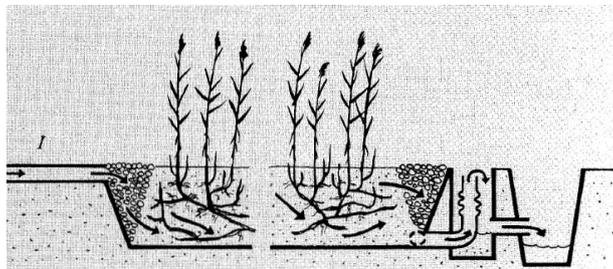
Figure 1: Constructed wetland with sub surface horizontal water flow. Consists typically of a bed planted with *Phragmites australis* and underlain by an impermeable membrane to prevent seepage. The medium in the bed may be soil or gravel.
