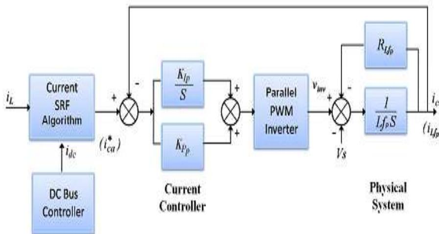
Fig. 2. SRF current control block diagram.
