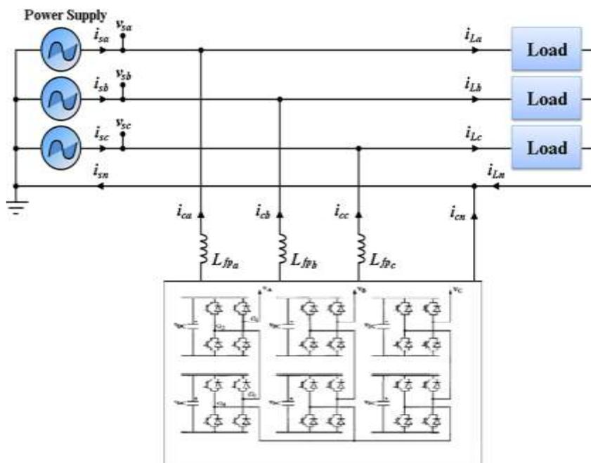
Fig.3 Proposed system circuit diagram
