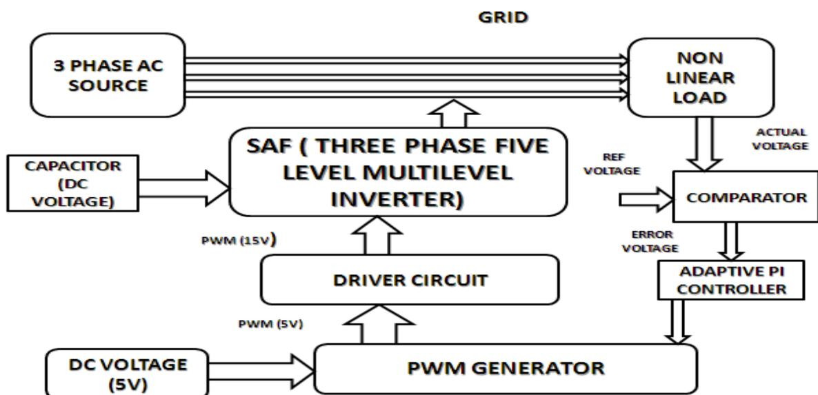
Fig. 1. Block diagram of the SAF system.
