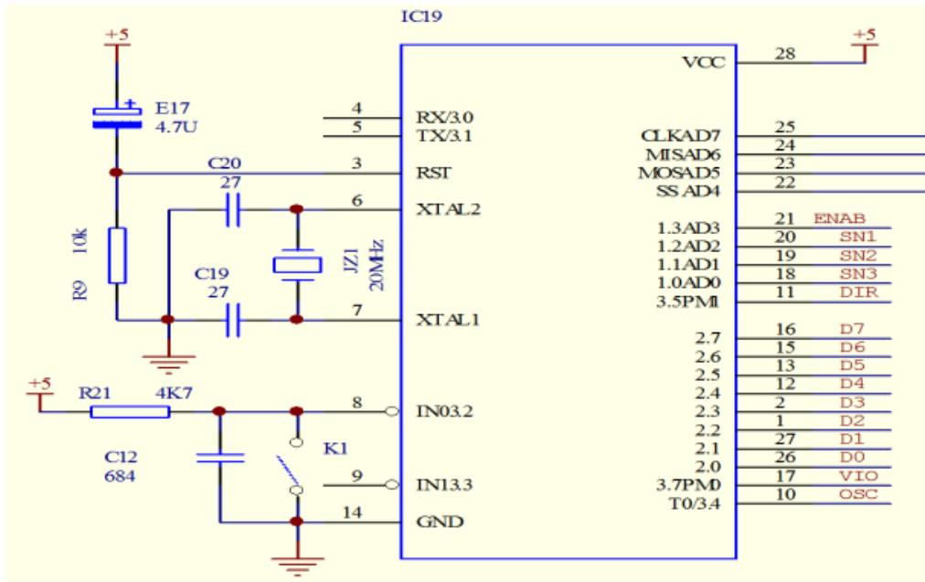
Figure 5. Single-chip microcomputer controlled circuit
