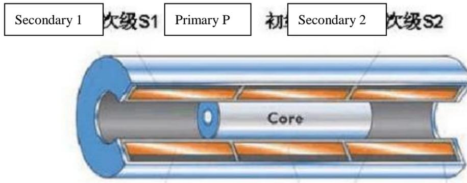
Figure 1. Structure diagram of LVDT
