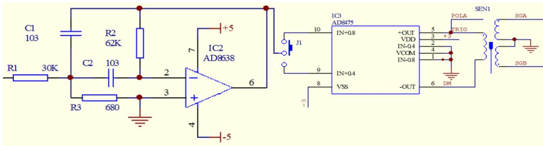
**Figure 3. Filter circuit and the driving circuit**
