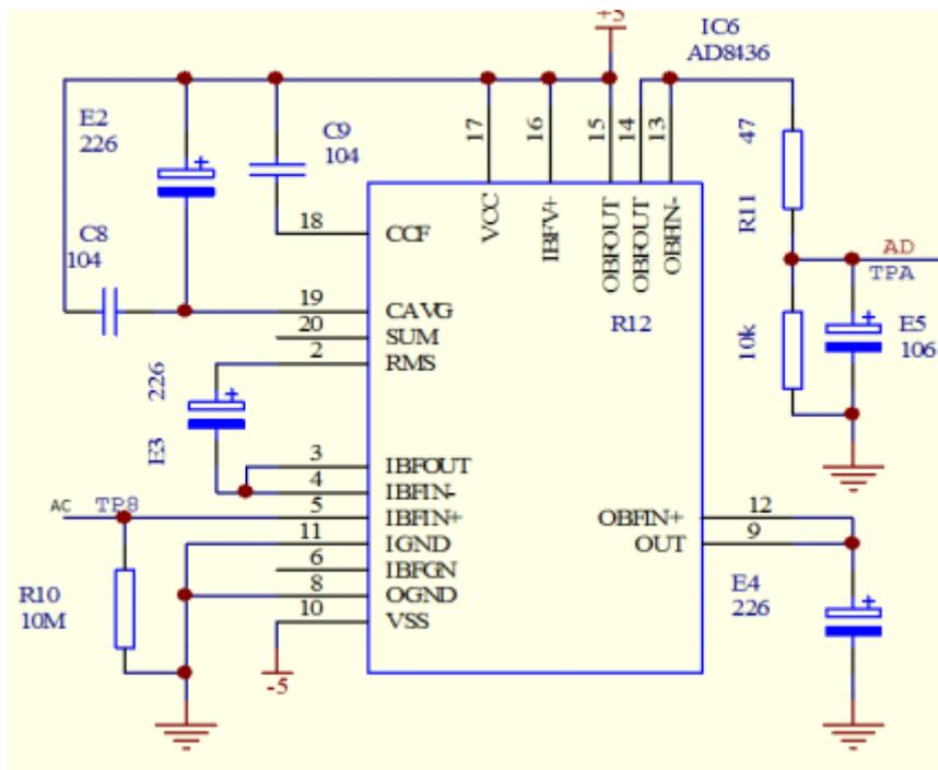
**Figure 4. Virtual value transformation circuit**
