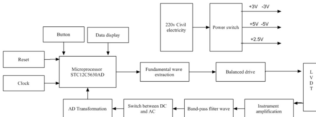
Figure 2. Structure diagram of this system
