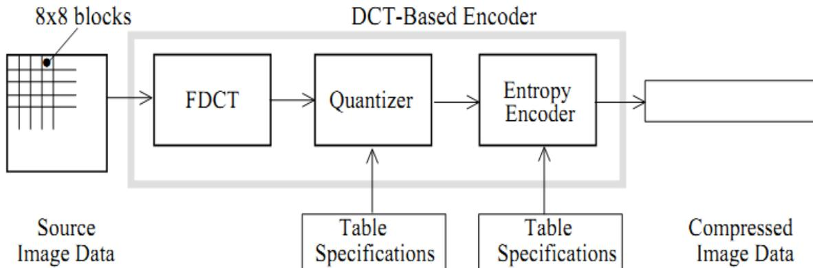
Fig (1) DCT Based Encoder
