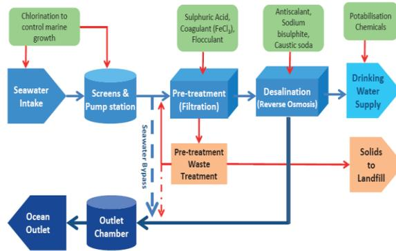
Fig 2- RO Desalination process (Source: Fichtner, 2011)
