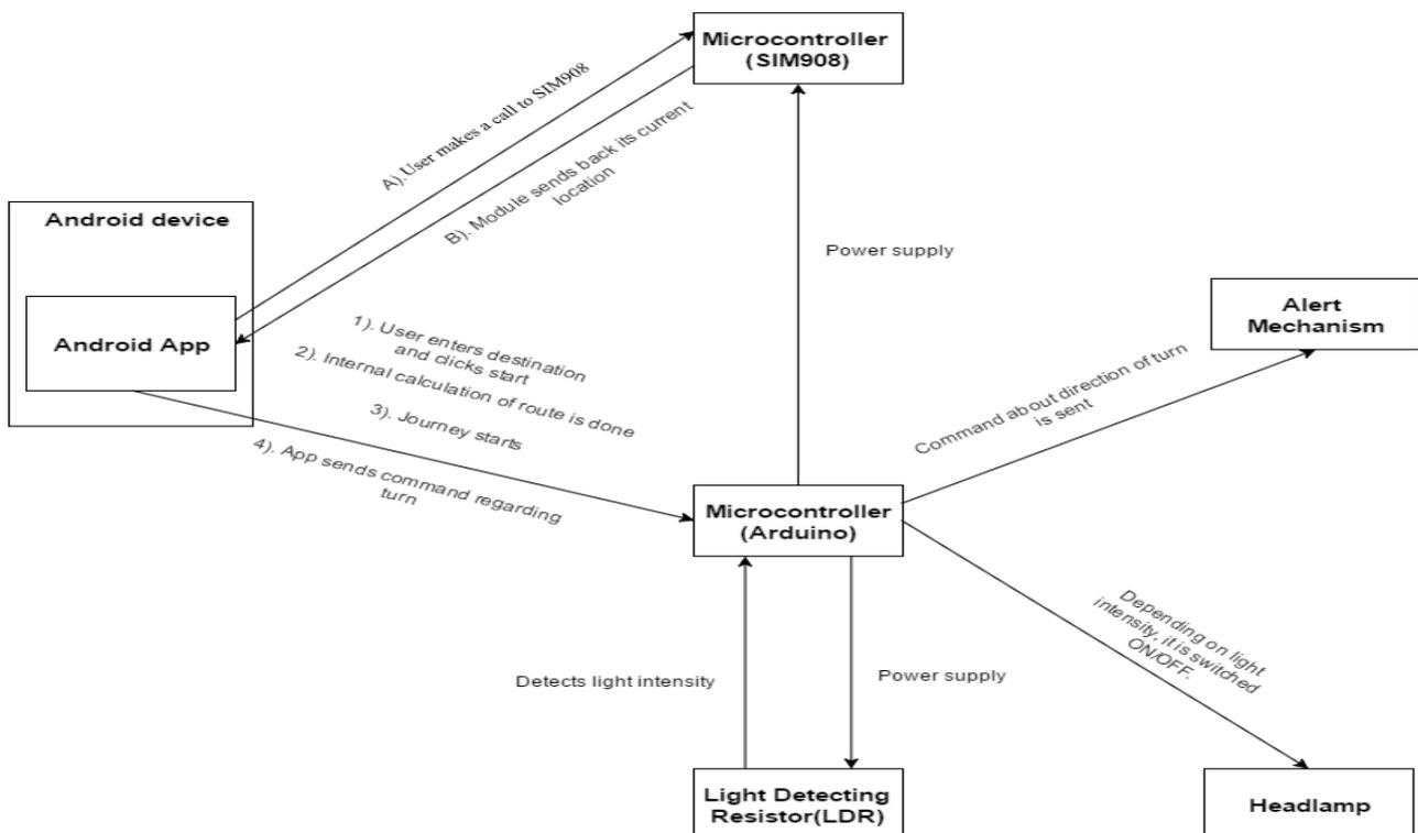
Figure 1. Process flow for smart bicycle.
