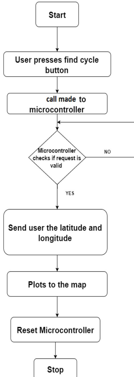
Figure 2. Flow diagram for vehicular tracking.
