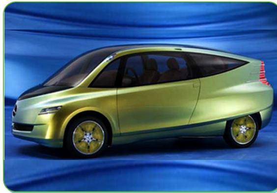
Figure 4: Appearance of Bionic car inspired by boxfish
