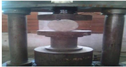
Fig.5 : Split tensile test on concrete cylinders
