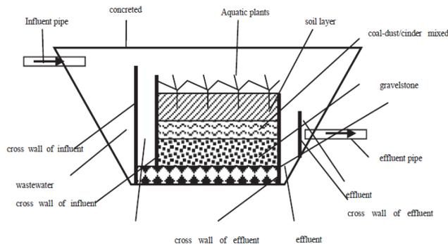
**Fig. 2 Structure of multilayer (Shibao Lu et al., 2015)**
