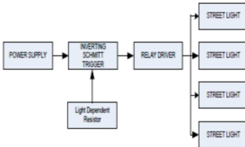
*Fig 3 Street Lighting System Using Schmitt Trigger*
