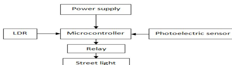
Fig 1. Block diagram of street Light system.
