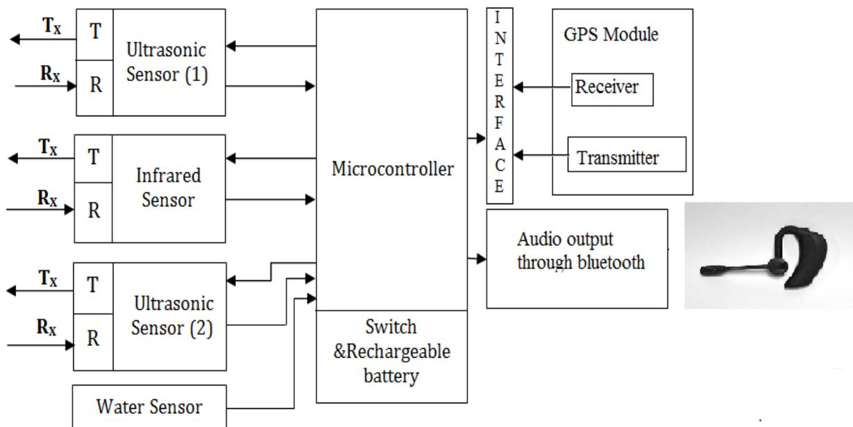
Fig. 1. Block diagram of Smart stick
