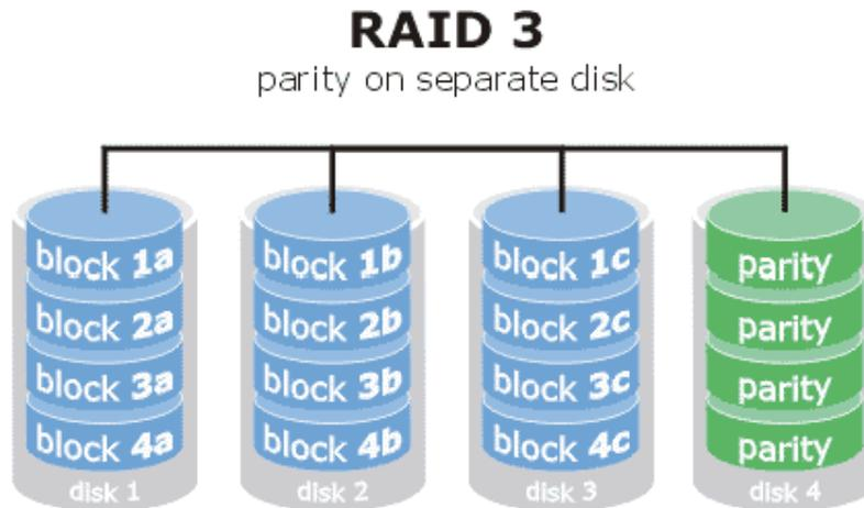
Since parity is used, a RAID 3 stripe set can withstand a single disk failure without losing data or access to data.
