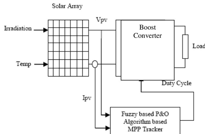
Fig. 8 Schematic Block Diagram of Proposed Power Conversion
