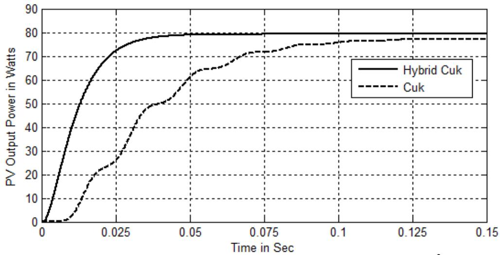
Fig. 13 PV Output Power at Solar Irradiation of 600 watts/m<sup>2</sup>
