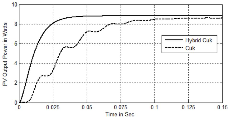
FIG. 11 PV OUTPUT POWER AT SOLAR IRRADIATION OF 200 WATTS/M<sup>2</sup>
