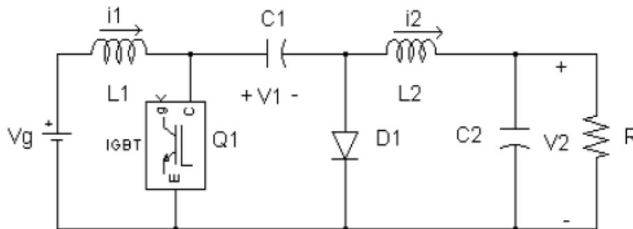
Fig. 6 Circuit diagram of Cuk Converter
