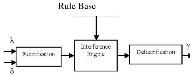
**Fig. 4 Four Basic Elements in Fuzzy Logic Controller**
