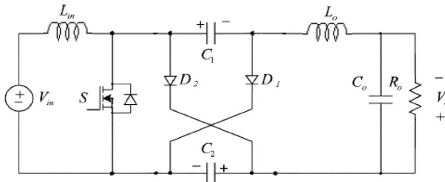
Fig. 7 Circuit diagram of Boost Boost Mode Cuk Converter
