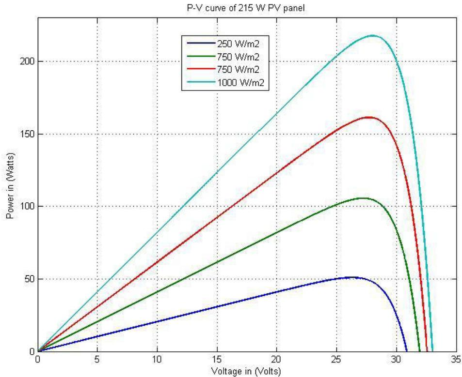
The main limitation of P&O MPPT approach is the PV module's operating voltage is troubled every cycle [18]. The algorithm will always carry out an increment or decrement of  $\Delta V$  to the PV operating voltage. The *process* of maximum power tracking will be executed on even the MPP has been effectively tracked. This is because of the output power of PV module for the next perturbed cycle is unpredictable.
