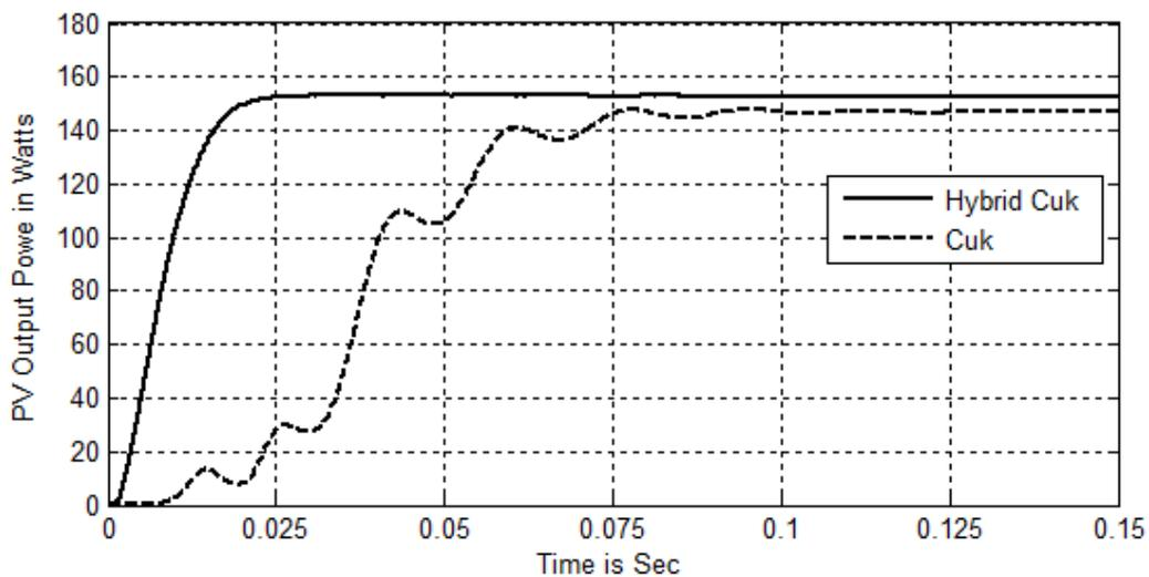
Fig. 15 PV Output Power at Solar Irradiation of 1000 watts/m<sup>2</sup>
