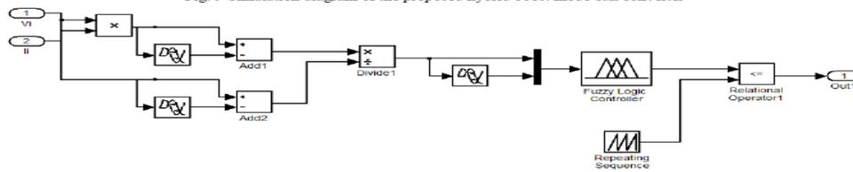
Fig. 10: Fuzzy logic based P & O algorithm in simulink
