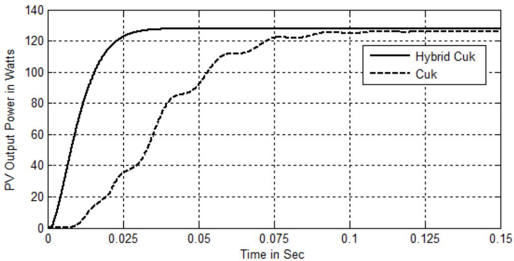
Fig. 14 PV Output Power at Solar Irradiation of 800 watts/m<sup>2</sup>
