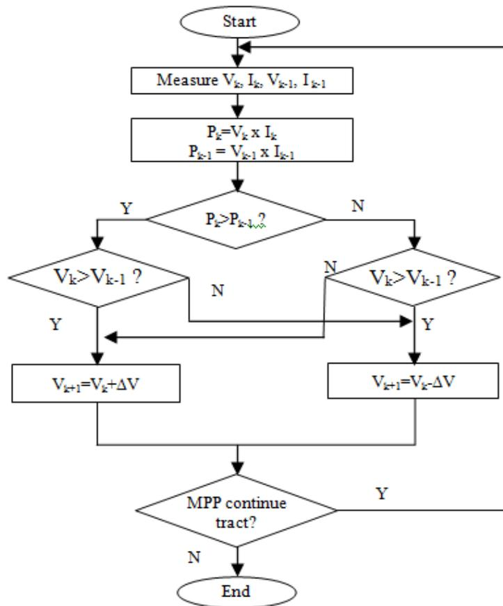
Fig. 2 Flowchart Shows the Operation of P&O MPPT
