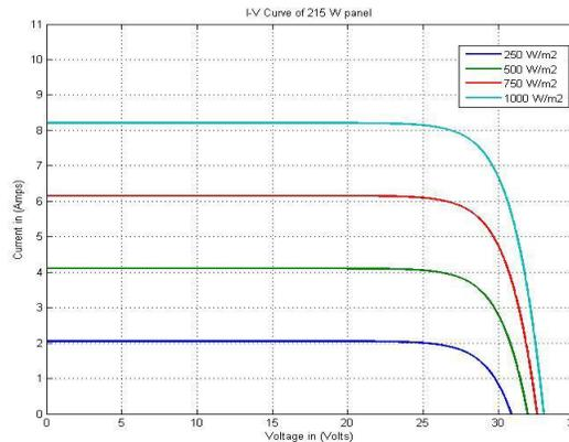
**Fig. 1 Current Vs Voltage Curve of a PV Module**
