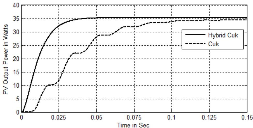
Fig. 12 PV Output Power at Solar Irradiation of 400 watts/m<sup>2</sup>
