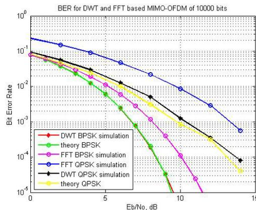
**Fig 5. BER vs Eb/No for FFT and DWT based MIMO-OFDM for 10000 bits**
