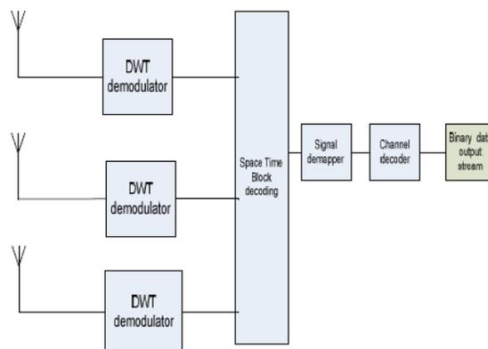
**Fig 4. Block diagram representation of DWT based MIMO-OFDM Receiver**
