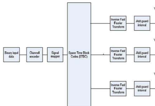
**Fig 1. Block diagram representation of FFT based MIMO-OFDM Transmitter**
