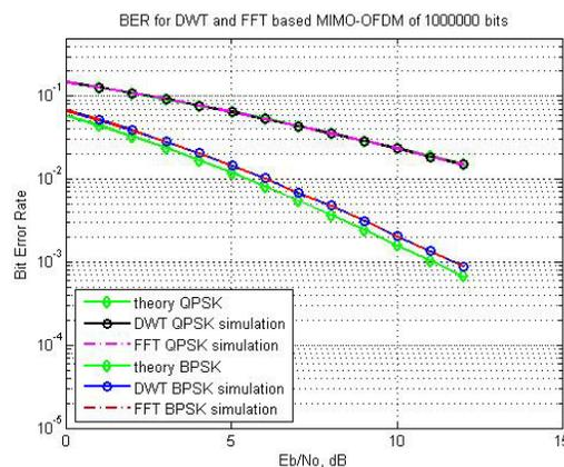
**Fig 6. BER vs Eb/No for FFT and DWT based MIMO-OFDM for 1000000 bits**
