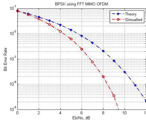
Fig 7. BER vs  $E_b/N_0$  for FFT based MIMO-OFDM for BPSK Modulation Scheme
