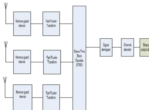
**Fig 2. Block diagram representation of FFT based MIMO-OFDM Receiver**
