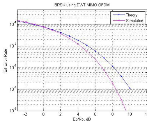
Fig 8. BER vs  $E_b/N_0$  for DWT based MIMO-OFDM for BPSK Modulation Scheme
