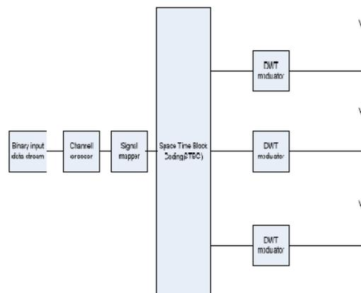
**Fig 3. Block diagram representation of DWT based MIMO-OFDM Transmitter**
