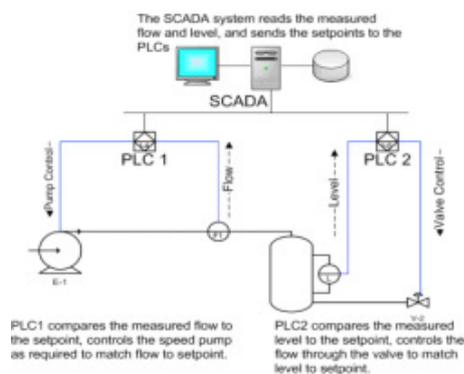
**Fig 4: SCADA Communication System**
