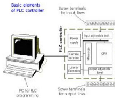
Fig 3: Interfacing of PLC
