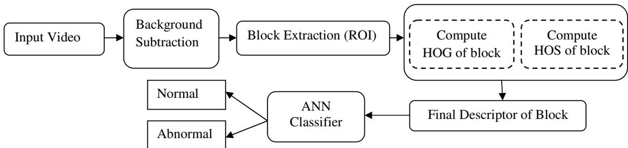
*Figure 1: The workflow of anomaly detection and classification*
