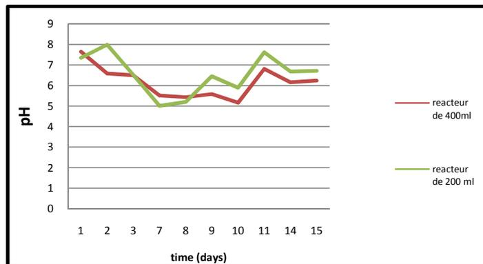
*Figure 2: Changes in pH during anaerobic for both digesters.*
