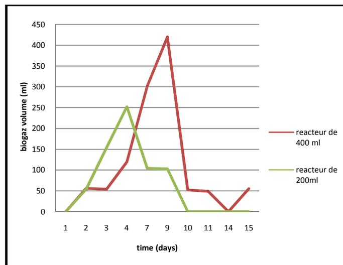
*Figure 3 : Daily production kinetics of biogas for both digesters.*
