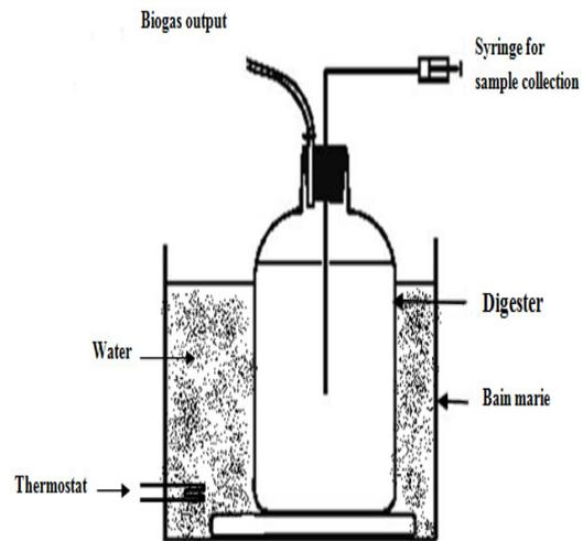
*Figure 1: Simplified diagram of the fermentation device used.*
