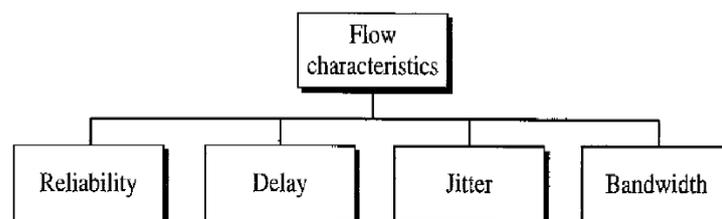
FIG 3. QoS FLOW CHARACTERISTICS
