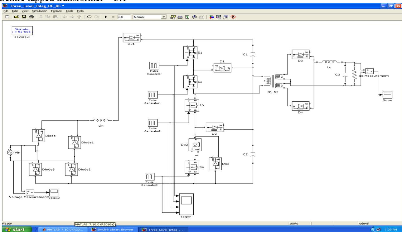
*Fig.6 Simulation of modified single stage ac-dc converter using Matlab/Simulink*
