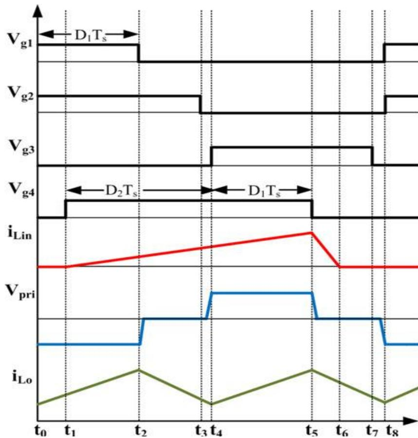
Fig. 3 Typical waveforms describing the switching modes of operation
