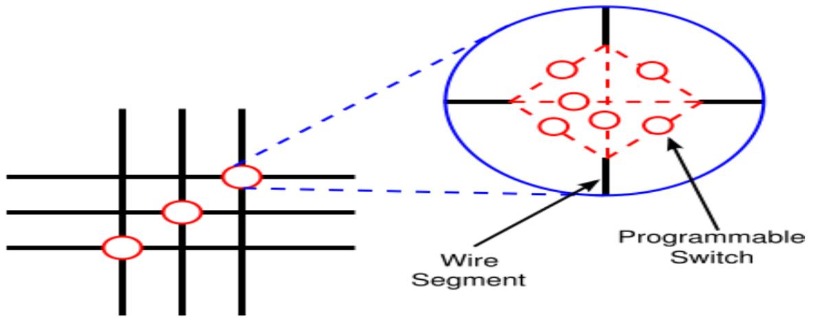
Fig.5. Switch box topology for FPGA controller
