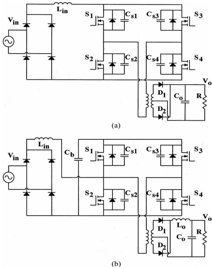
Fig. 1 Varies power factor correction single stage converter. (a) Boost based current fed ac-dc PWM integrated full bridge converter. (b) Power factor correction PWM full bridge converter.
