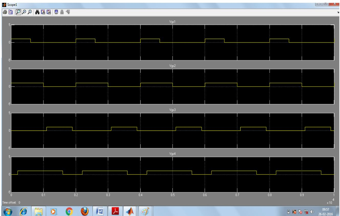
Fig.8 Simulation of switching waveforms for modified ac-dc converter
