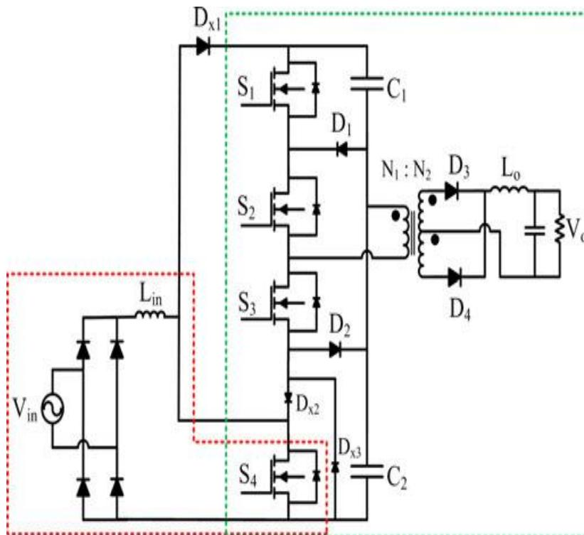
Fig. 2 modified single stage ac-dc converter
