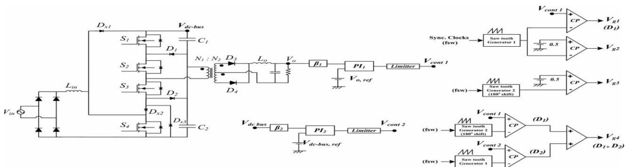
*Fig.4. Simplified schematic control of ac-dc converter*
