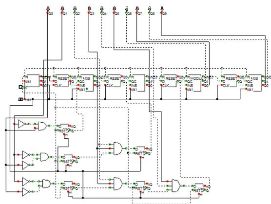
**Fig3.5: Schematic of High Speed 10 BIT Parallel Counter**
