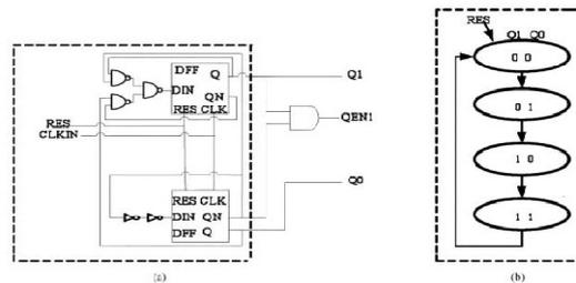
**Fig 2.2: Module-1 (a) Hardware schematic and (b) State diagram. Note that the 1 in QEN1 denotes that this is the QEN for module-1.**
