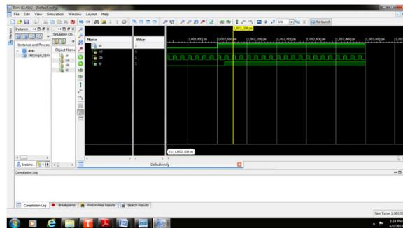
**Fig 3.1: Behavioral Simulation waveform for D-Flip Flop.**
