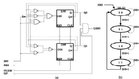
**Figure 2.3: Module-3S (a) hardware schematic and (b) state diagram.**
