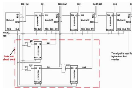
**Fig 2.1: Functional block diagram of the proposed 8-bit parallel counter with state look-ahead logic and counting logic.**
