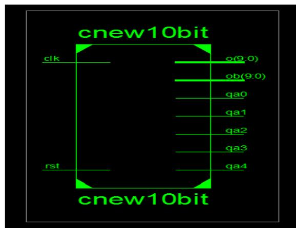
**Fig3.4: Parallel Counter Architecture Based on State Look-Ahead Logic symbol.**
