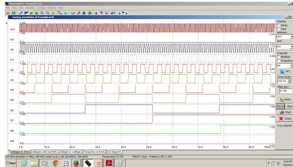
**Fig3.6 (a): Simulation result in 10 BIT Parallel Counter using DSCH Tool**
