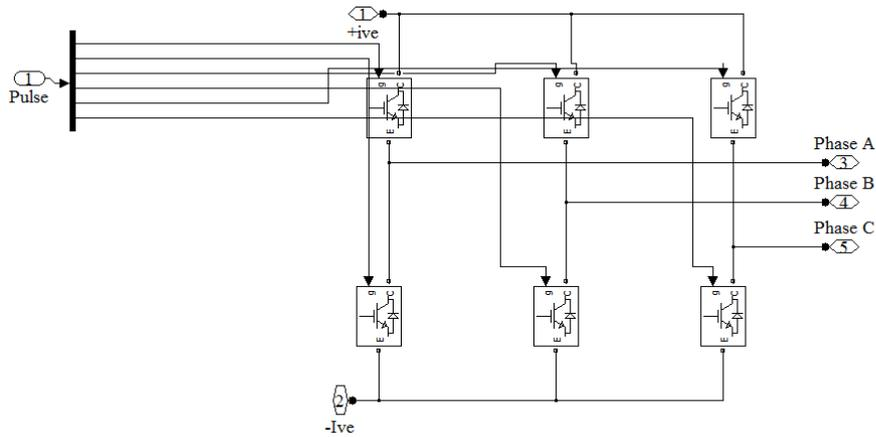
Figure 7. Matlab Simulink diagram for UPFC shunt converter
