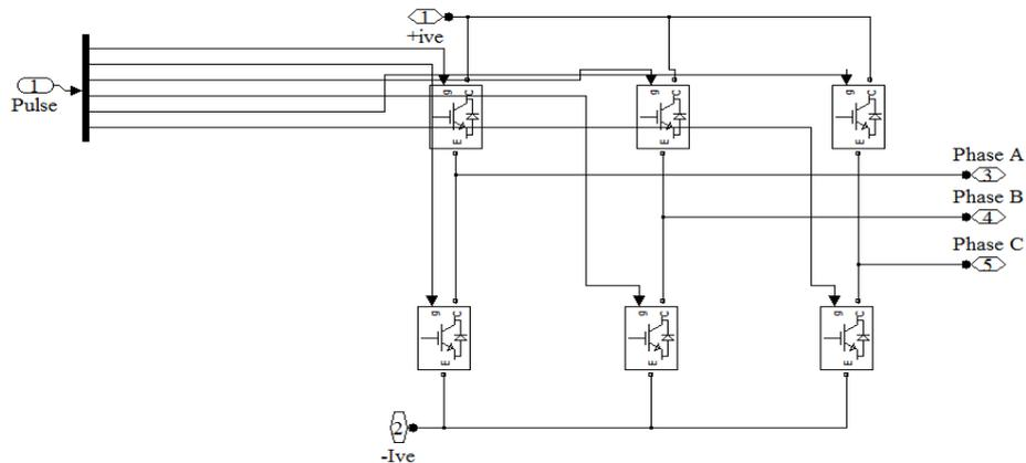
Figure 6. Matlab Simulink diagram for UPFC series converter
