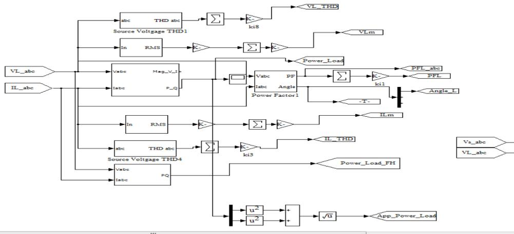
Figure 8. Matlab Simulink diagram for UPFC reference current generation
