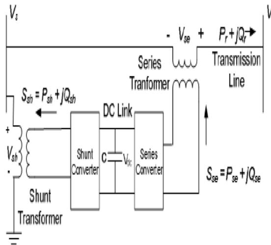
Figure 2. UPFC schematic diagram
