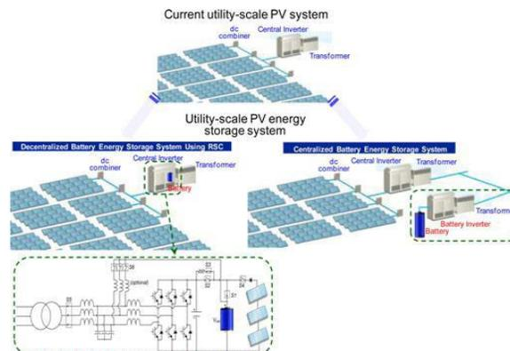
**Fig4. Utility-scale PV-energy storage systems with the RSC and the current state-of-the-art solution.**
