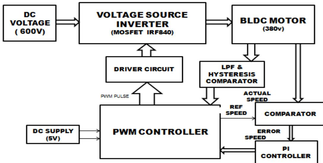
Fig 1. Block diagram of Sensorless BLDC motor
