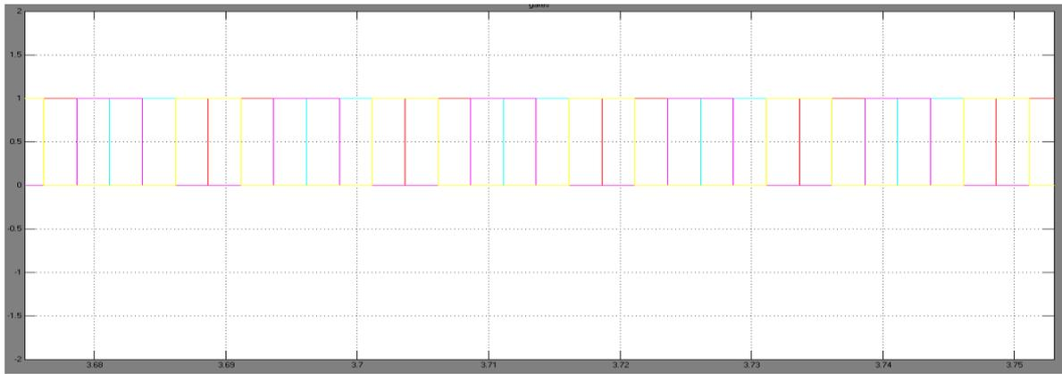
*Fig.9. Gate pulses to the inverter*
