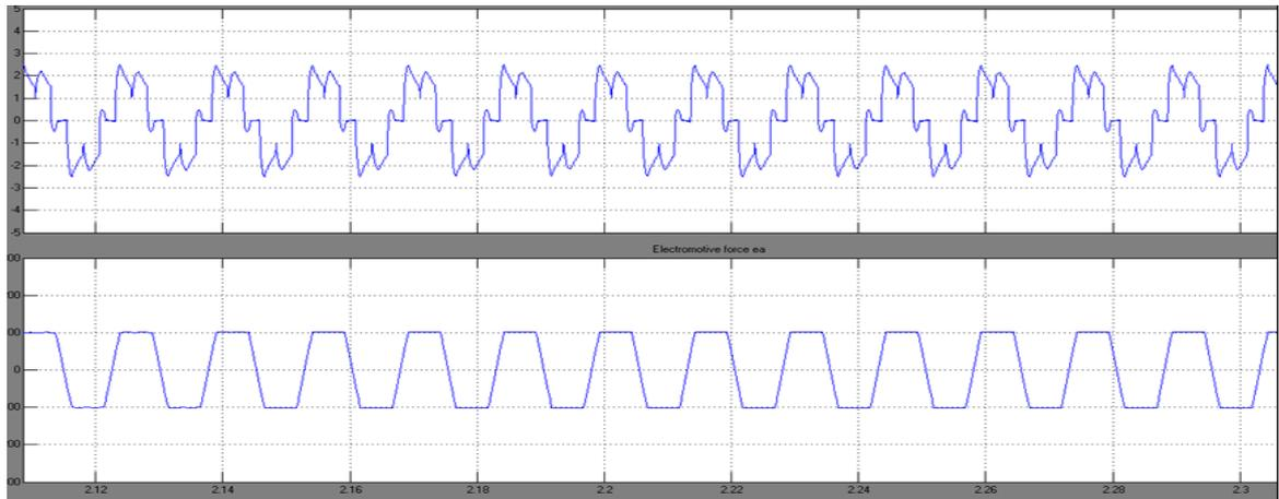
Fig.7. Three phase voltage source inverter output and back emf waveform of BLDC motor
