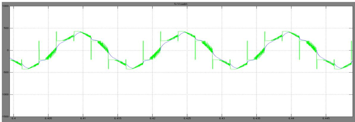
Fig.8. Back emf waveform before and after filter
