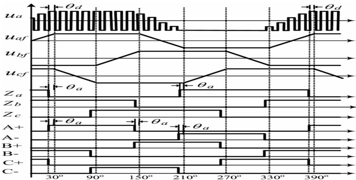
Fig 4. Hysteresis comparator output
