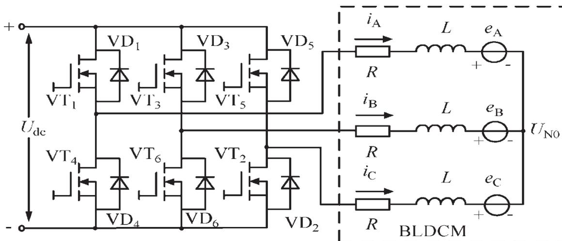
Fig 2. Circuit diagram of Sensorless BLDC motor
