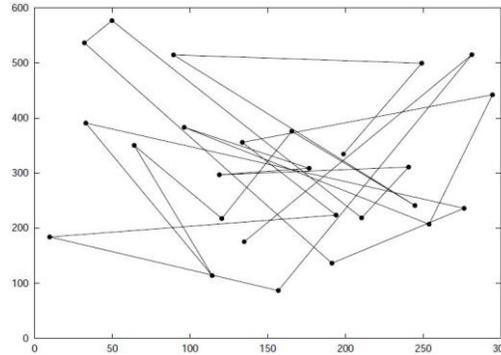
**Figure 4. Travelling Pattern of an MN using the Random Waypoint Mobility Model [7]**
