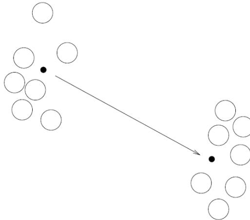
*Figure 8. Movements of seven nodes in Nomadic Mobility Model [9]*
