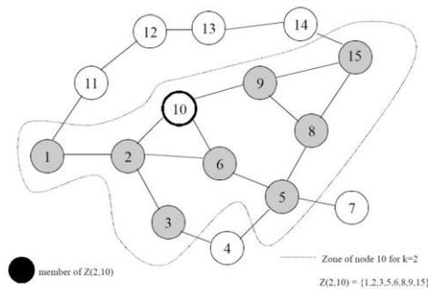
**Figure 3: ZRP Routing Protocol [2]**
